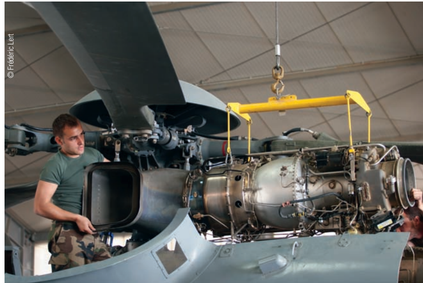
Maintenance performed on EC725s in Kabul is largely preventive, and based on the same maintenance intervals for civil helicopters.
