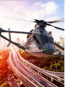
The configuration of the "Racer" high-speed demonstrator rotorcraft was unveiled at the Paris Air Show. Developed as part of the Clean Sky 2 European research programme, it would have a cruise speed of over 400 km/hour.
