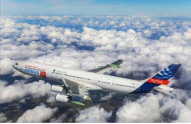
**Airbus' A340 laminar flow "BLADE" test demonstrator aircraft** made its successful first flight. Part of the EU-sponsored Clean Sky "BLADE" project, the technology aims to reduce wing friction by 50% and  $\mathrm{CO_2}$  emissions by up to 5%.
