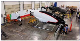
In 2017, **the Vahana urban air mobility vehicle** was assembled and underwent ground tests. This revolutionary, self-piloted vertical take-off and landing (VTOL) passenger vehicle flew for the first time in January 2018.
