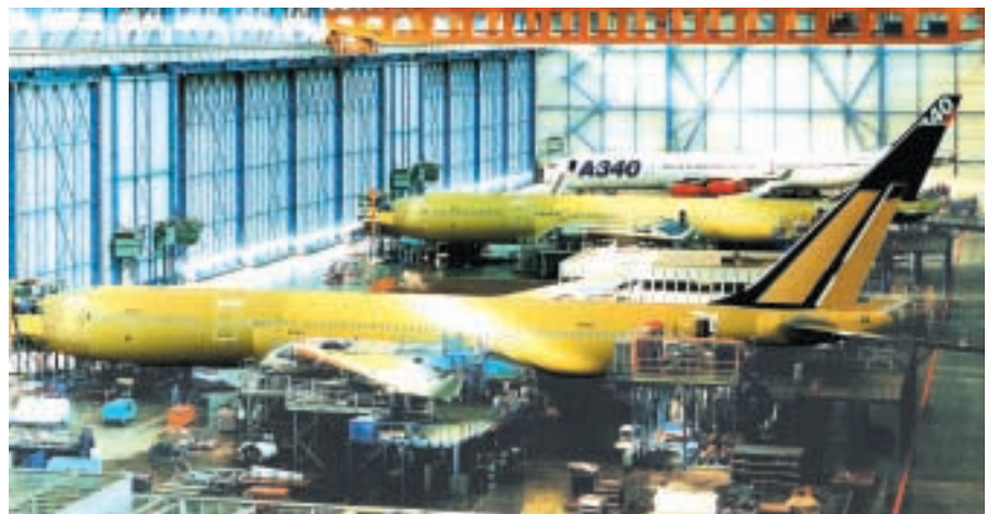
A330 and A340 final assembly line
