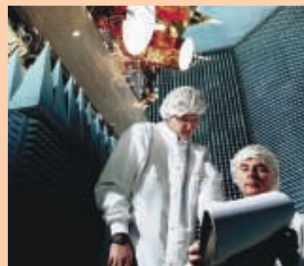
Envisat is placed in an Astrium anechoic chamber to check compatibility of the various radio frequencies
