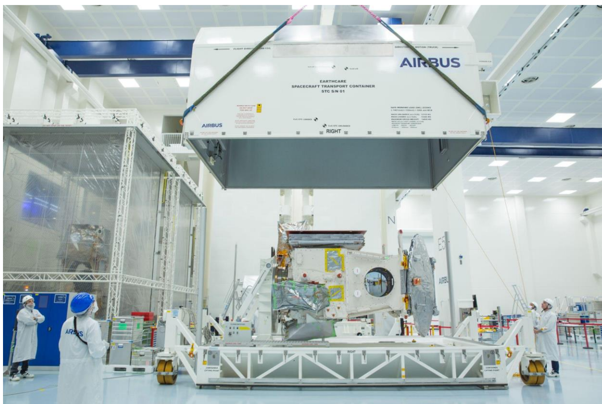
EarthCARE satellite is packed into its container for its flight to launchpad - Copyright Airbus
