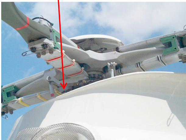
Possible access for extinguishing
