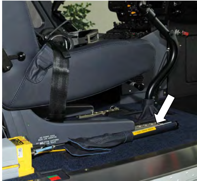
Rotor brake lever is located beside the Pilot seat
